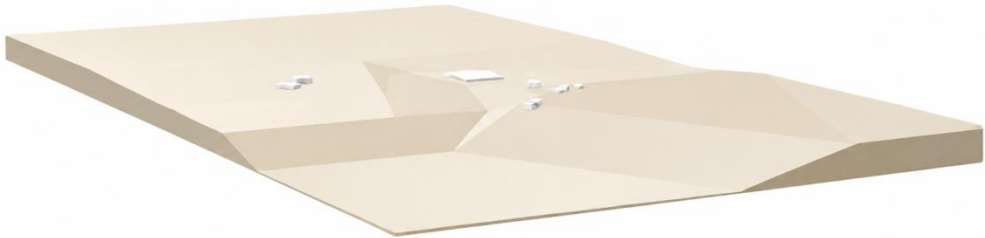
Fig. 3b. Manual terrain reconstruction in dBmap: three-dimensional terrain model obtained through triangulation.
