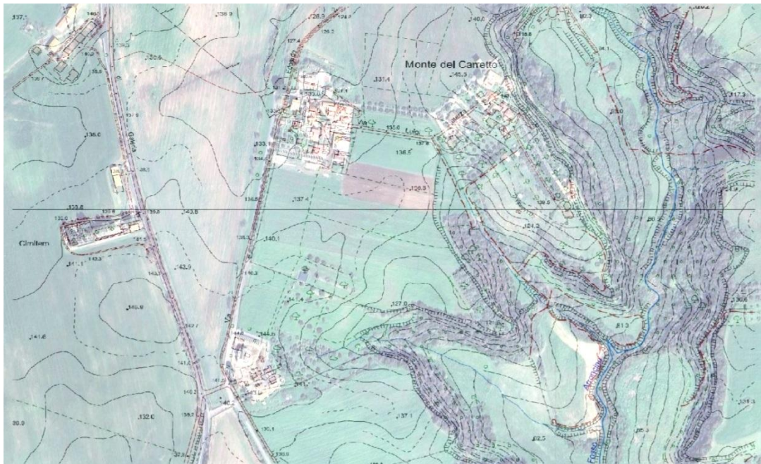
Fig. 3a. Manual terrain reconstruction in dBmap: georeferencing of elevation points on the cartographic base map (EPSG: 6708).
